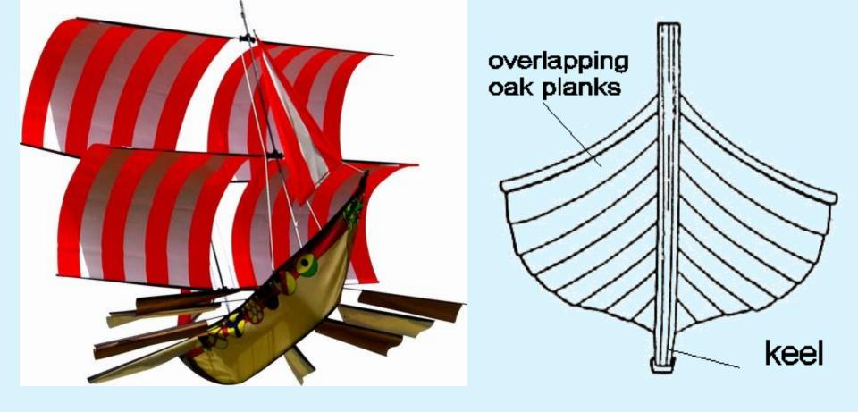
Viking longships were among the first ever ships to have a keel. The keel is extremely important as it provides the ship with support in rough weather.
